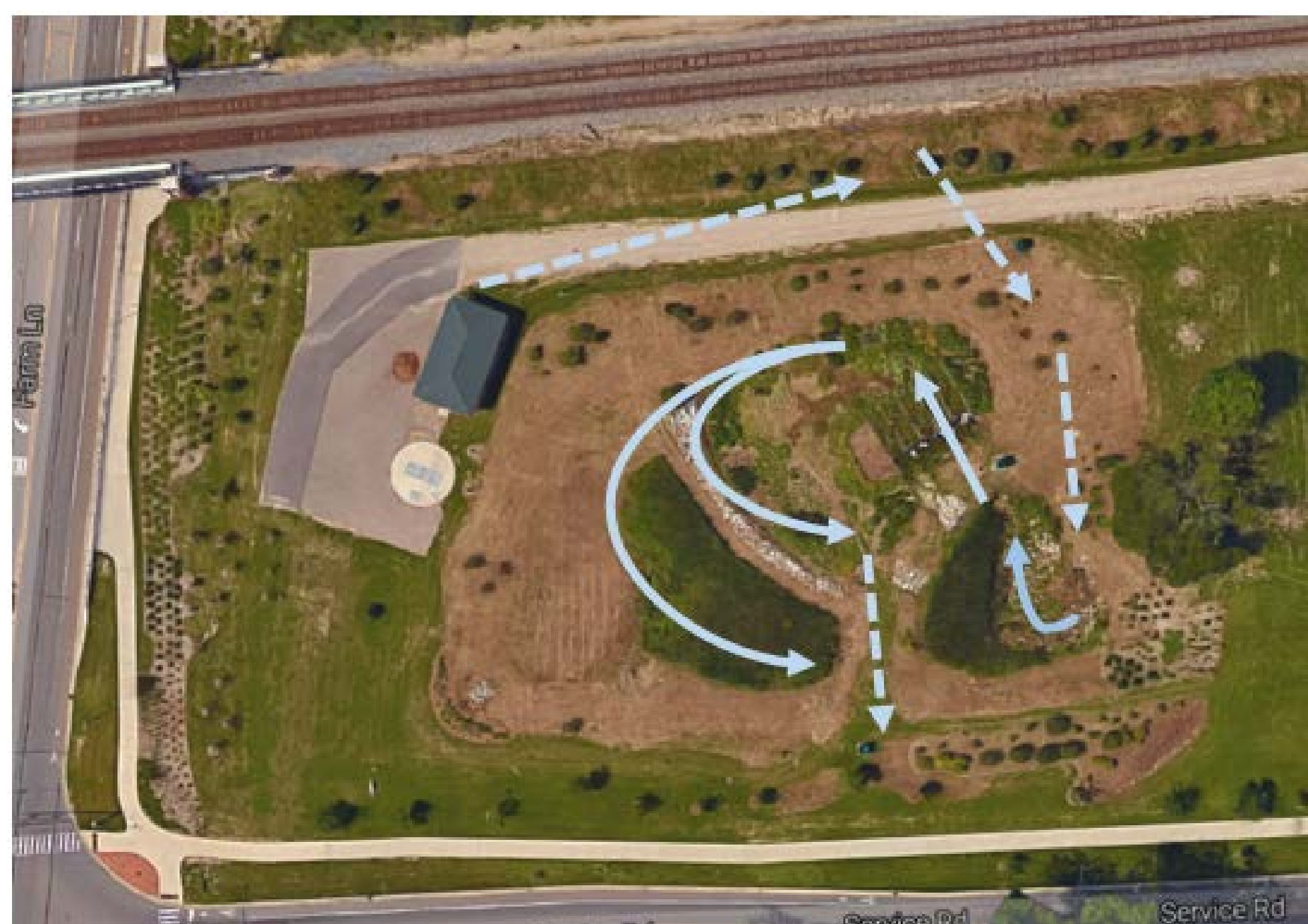
Figure 1: Farm Lane Bioretention Basin and Flow Map
