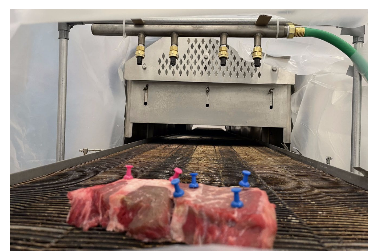
Figure 3: Beef sample with indicated swabbing sites within isolated spray chamber
