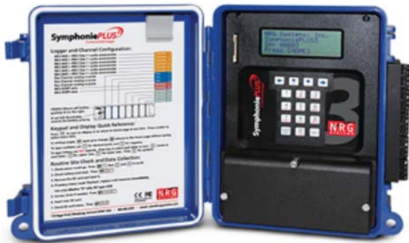
Figure 10. Example of a met tower data logger.
