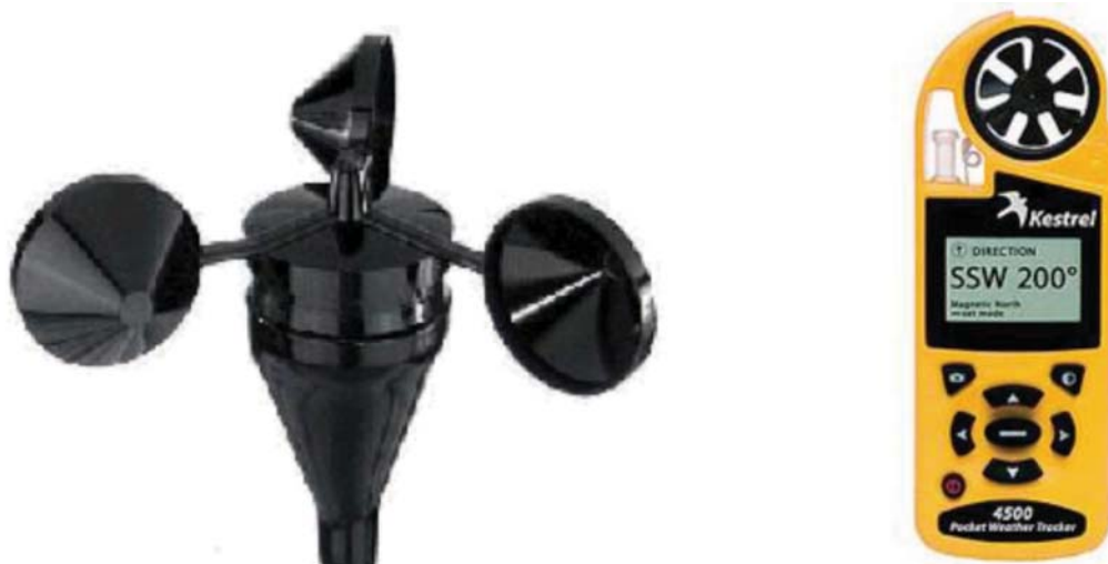
Figure 8. Example of a vertical-axis anemometer (left) and horizontal-axis anemometer (right) Source: Vertical axis anemometer, NRG Systems, www.nrgsystems.com ; horizontal-axis anemometer, Kestrel Meters, www.kestrelmeters.com
