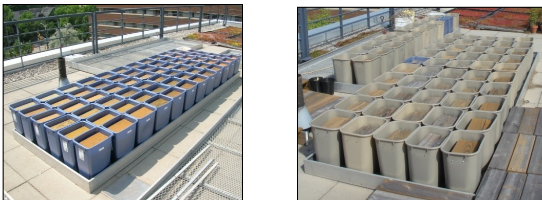
Figure 2.1: Natural weathering samples before and after 3 years of exposure.
