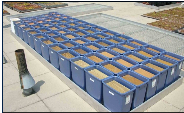
Figure 5.1: Natural weathering setup- Treated coated and uncoated samples were exposed to natural weathering, in Toronto, Canada
