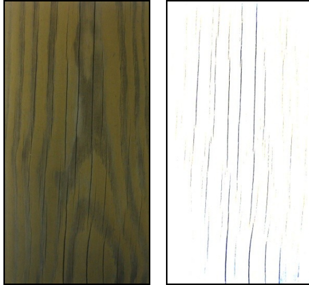
Figure 2.2: (left) Sample after 3 years of natural weathering and (right) evaluated by image analysis for checks area measurement
