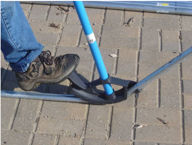
12' wide, 12' long, ~ 7' tall; 10' long 1" diameter EMT conduit bent at 45° and joined at top. Exterior joining spline and ground posts made with 1.3" chain link fence top rail.
