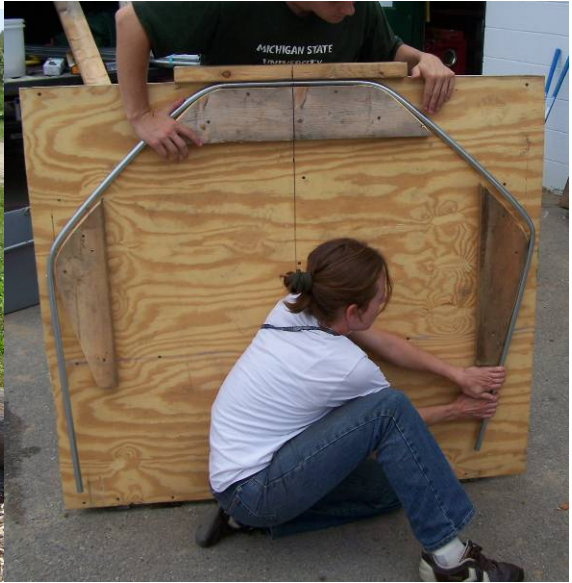
Mini greenhouse cold frame from 1/2" EMT and wire lock channels to hold plastic; jig to bend conduit.
