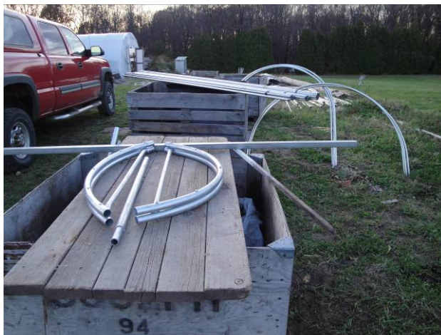
1/2" EMT 4' and 6' quick hoop bender from Johnny's Seeds and three, 60° bends with conduit bender. Takes about the same amount of time; could make a jig like the one above.
