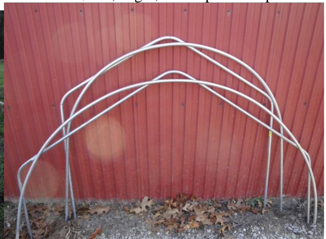
1/2" EMT 4' and 6' quick hoop bender from Johnny's Seeds and three, 60° bends with conduit bender. Takes about the same amount of time; could make a jig like the one above.
