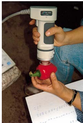
Measuring fruit surface color using a colorimeter
