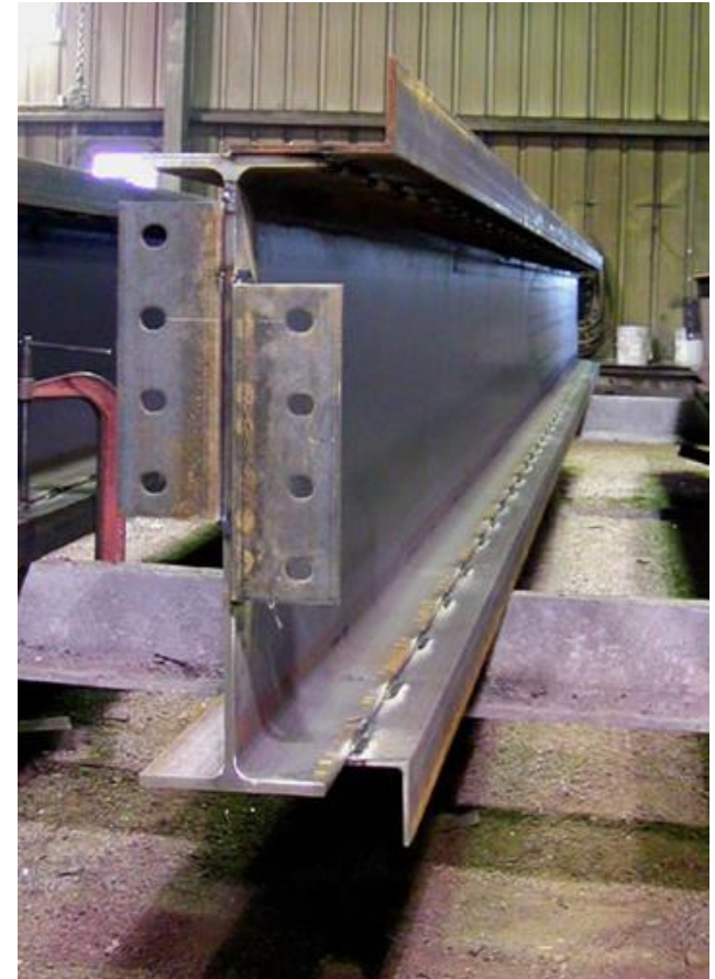
Fabricated beam with connection work
