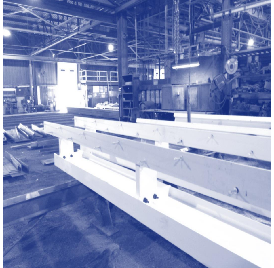
Fabricated elements ready for shipping
