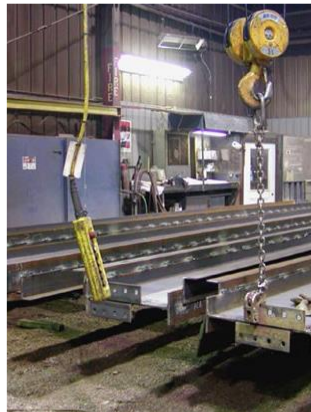
Overhead crane used to move material in shop
