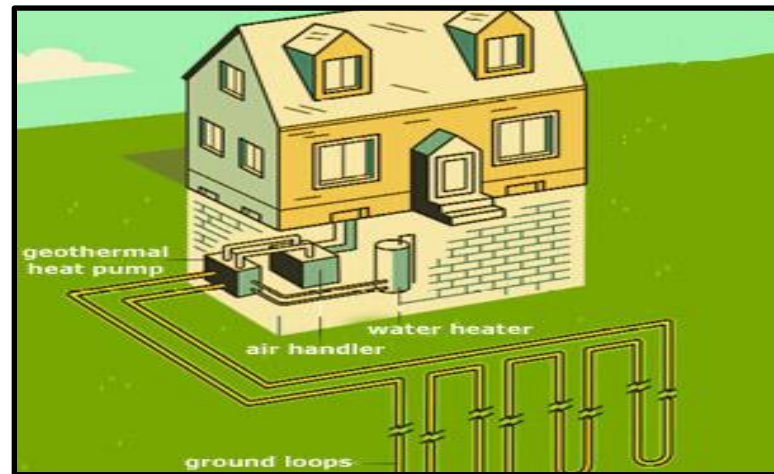
FIGURE 28: Geothermal System Diagram; Source: http://climateprogress.org/2008/08/07/the-other-geothermal-grew-33-in-2006/
