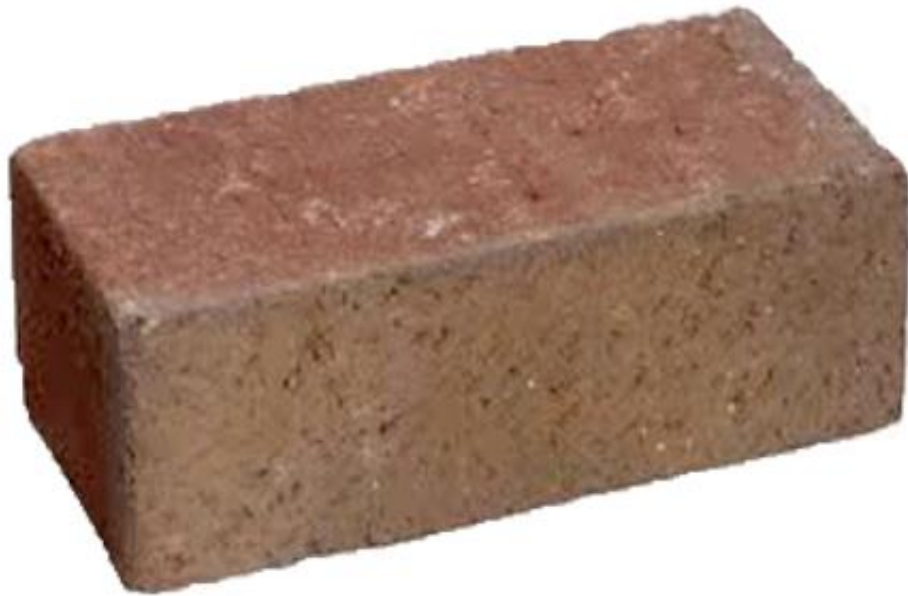
Brick = high bulk density, low pore space
