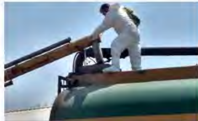
Figure 3. Collection of bioaerosol during manure pump-out with filter media approximating the top of the fill-port at the point of dispersion of pathogen containing bioaerosol will disperse via laminar air movement.
