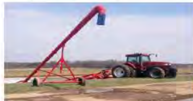
Figure 4. Positioning of tractor and swing arm for earthen storage (lagoon) pump-out. Note substantial puddling on drive potentially resulting in pathogen transport via vehicle(s) and human (foot) traffic.
