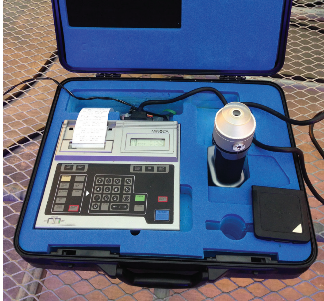
Figure 2. The colorimeter is a non-destructive instrument used by the U.S. food industry for measuring and tracking color changes of fruits and vegetables during processing and storage. In our study, we used the colorimeter to determine and track lettuce leaf color without damaging leaves or plants.
