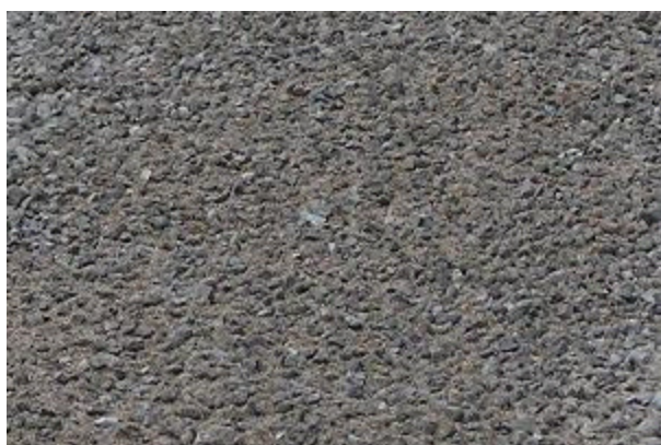
Figure 3. Typical extensive green roof medium.
